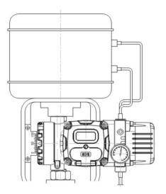
Figure 4-3 Double acting type linear actuator
