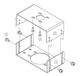
Figure 3-9 : Bracket set for rotary positioner installation
