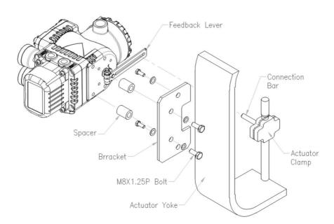
Figure 3-2 : SP760 positioner installation in actuator
