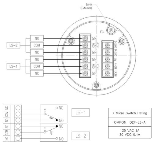
Figure 5-3 : Limit switch connection map
