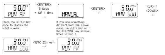
The numbers of the 2nd row indicates the target position and MAN 300 shows 30.0 % in the captioned picture.
