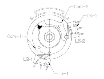
Figure 6-1 : Adjustment of limit switch operation
