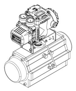
Figure 4-2 : Single acting rotary actuator
