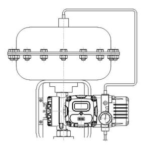
Figure 4-1 Single acting linear actuator
