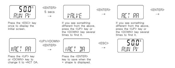
\* This work must be done after shut down air or 50% position condition. In this time ,actuator shall be operated reversely .
