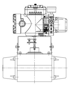
Figure 3-7 : Fork Lever type installation
