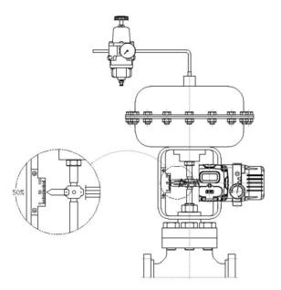
Figure 3-3 : SP760 positioner installation in actuator
