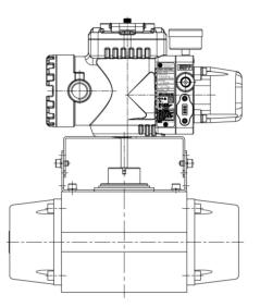
Figure 3-7 : Namur type installation
